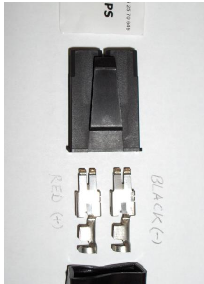
Picture A: interface: operation board to controller device and adapter. Attention: Please look for the right colours!
